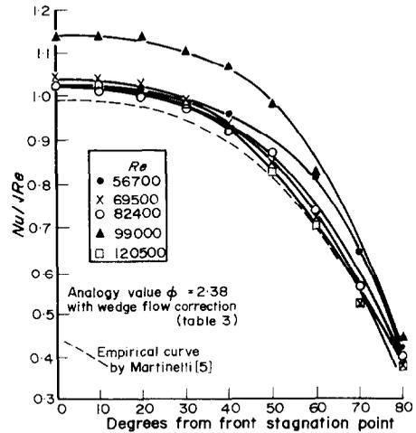
FIG. 2. Nu and erosion rate around cylinder periphery.
