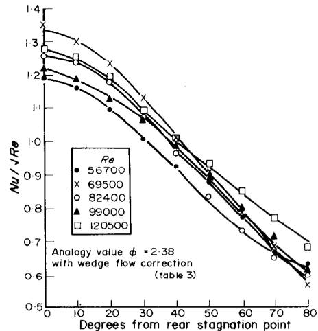
FIG. 6. Values from mass transfer experiments around the rear stagnation point.
